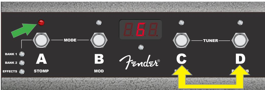
To activate the footswitch tuning function, step on buttons "C" and "D" simultaneously (double yellow arrow). In the example above, a "G" note is displayed as being particularly flat, as indicated by the illumination of the red LED above button "A" (green arrow).
