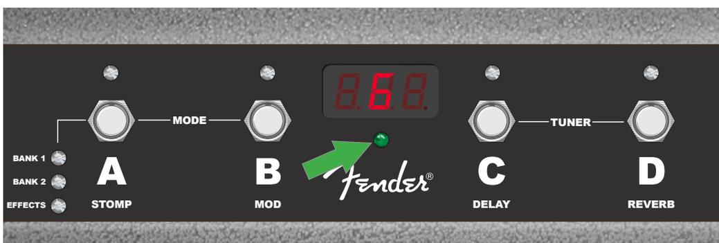
Here, the "G" note is at correct pitch, as indicated by the illumination of the green center LED (green arrow). When tuning is complete, step on any button to exit footswitch tuner mode.
