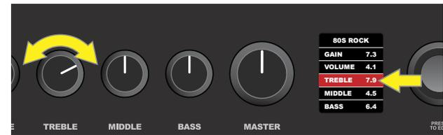
At this point, press the ENCODER or the BACK utility button (green arrow) to accept the adjusted control values. Pressing BACK returns the user to the preset contents screen; pressing the ENCODER lets the user continue making controls setting changes, and the box surrounding the control setting will return to blue. When control setting edits are complete, press the SAVE utility button to save the changes to the preset.
