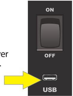
Note that although the USB port and the auxiliary input *can* be used simultaneously, the USB port *cannot* be used to record a signal from the auxiliary input. Also note that the USB output is in stereo, and that while preset gain, volume and tone controls will affect USB level and tone, the MASTER VOLUME control does *not*.
