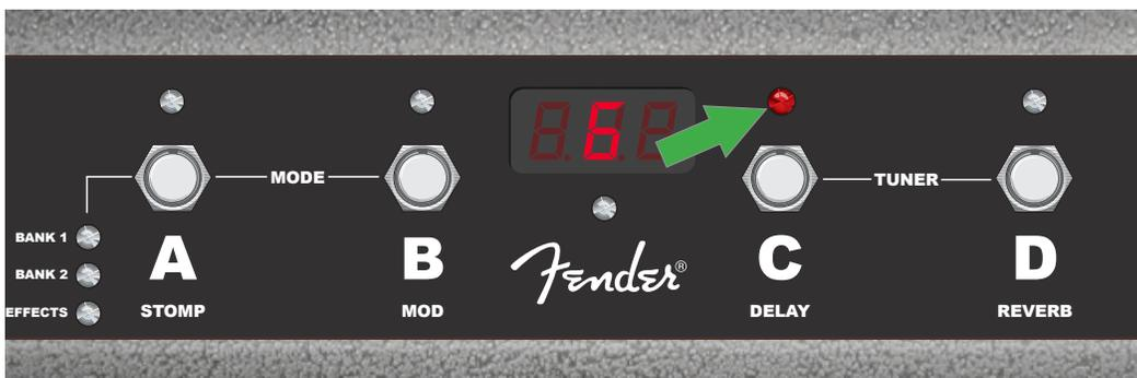
Here, the "G" note is displayed as slightly sharp, as indicated by the illumination of the red LED above button "C" (green arrow).
